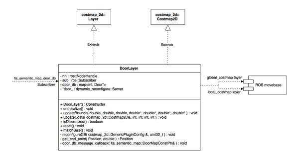
Figure A.2.: Classdiagram of the DoorLayer class of the costmap component.
