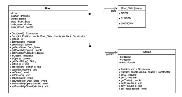
Figure A.3.: Classdiagram of the Server data classes.
